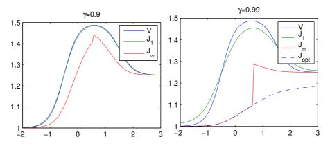
**FIGURE 3.** The policy improvement algorithm, that computes iteratively the value of a policy and then defines a new policy that is greedy with respect to this value function. In each figure, we show V(x), the value  $(1 - \gamma)J_1(x)$  of the random initial policy, and  $(1 - \gamma)J_{\infty}(x)$  the value of the converged policy, all as a function of *x*.
