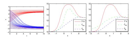
**FIGURE 5.** Left: Trajectories  $x_{1:n}^*$  that minimize the Action Eq. 26 used in the Laplace approximation. T = 10, R = 1. Time discretization dt = T/n, n = 10. Middle: Optimal cost-to-go J(x) for different x using the Laplace approximation ( $J_{lp}$ , dashed line) and the MC sampling ( $J_{mc}$ , dashed-dotted line) for v = 0.01. Right: idem for v = 1.
