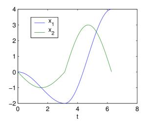
**FIGURE 1.** Optimal control of mass on a spring such that at  $t = 2\pi$  the amplitude is maximal.  $x_1$  is position of the spring,  $x_2$  is velocity of the spring.
