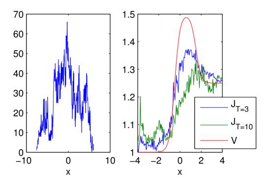
**FIGURE 6.** Sampling of J(x) with one trajectory of N = 8000 iterations starting at x = 0. Left: The diffusion process Eq. 33 with f = 0 explores the area between x = -7.5 and x = 6. Shown is a histogram of the points visited (300 bins). In each bin x, an estimate of  $\psi(x)$  is made by averaging all  $\psi(x_i)$  with  $x_i$  from bin x (not shown). Right:  $J_T(x)/T = -v \log \psi(x)/T$  versus x for T = 3 and T = 10 and V(x) for comparison. Time discretization dt = 0.02, v = 1, R = 1.
