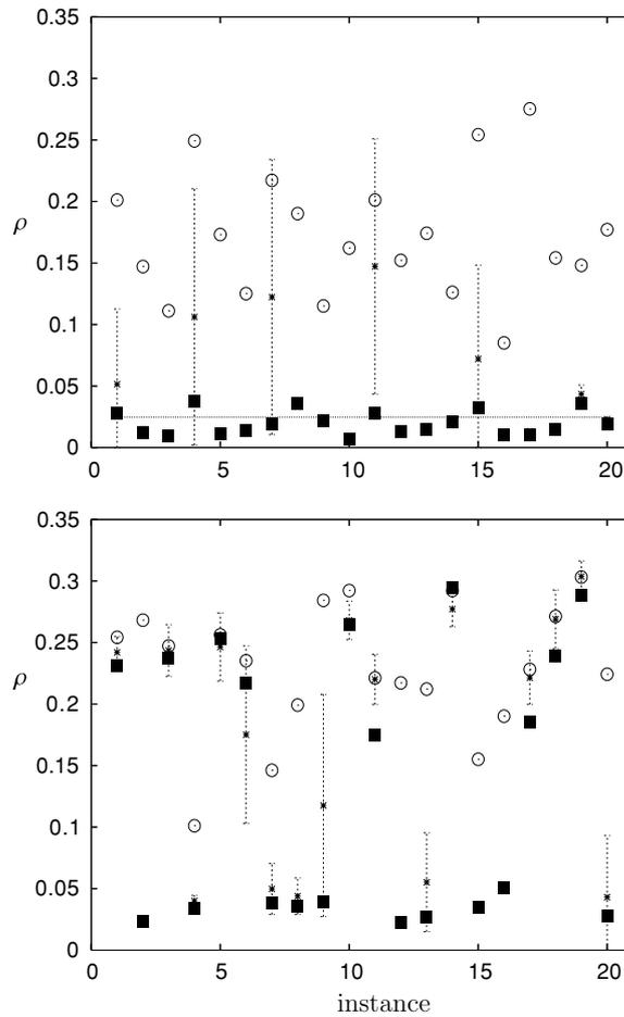
**Figure 3.**  $k = 4, \beta = 5$  single-instance bit error rate results for 20 systems of size  $N = 999$ , with channel noise  $p_{\text{ch}} = 0.07$  (top)  $p_{\text{ch}} = 0.08$  (bottom). Open circles: double-loop algorithm, full squares: our 1RSB algorithm, stars with error bars: ten runs of damped TABP, full square fall on top when not visible. Top figure horizontal line: population dynamics (ferromagnetic initial conditions) RS result.
