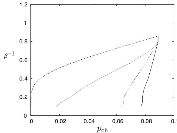
**Figure 2.** Replica symmetric phase diagram of the finite connectivity Sourlas code for  $k = 4$ ,  $p = 3$ ,  $c(0) = 0.8$ ,  $c(+) = c(-) = 0.1$ ,  $\theta = 1.5$ . From top to bottom the lines indicate the Nishimori temperature, the dynamic transition, the RS critical transition and the line along which the population dynamics algorithm ceases to find the ferromagnetic state.
