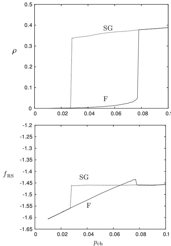
**Figure 1.** Top: bit error rate  $\rho$  as a function of channel noise for a code with  $k = 4$ ,  $\beta = 5$  and bias  $\theta = 1.5$  with ferromagnetic initial conditions versus spin-glass initial conditions. Bottom: the RS free energies corresponding to the top picture. In both figures the label F denotes ferromagnetic initial conditions and SG denotes the branch with spin-glass-type initial conditions (see text).
