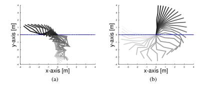
**Fig. 6.** Illustration of the estimated swing-up movement with the quad link. (a) time steps 1 to 35. (b) time steps 36 to 70. Lighter colors indicate an earlier time step.
