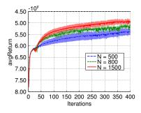
Fig. 5. Learning curve for the quad-link. An increasing number of samples always increases the performance.
