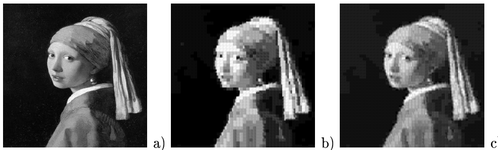
Figure 10. a) The Vermeer image prior to compression consists of 865 kbits. After compression: b) With standard vector quantisation I_v = 74 kbits, c) with GVQ using 1 set of 8 features (see fig(11)) I_{GVQ} = 56 kbits.
