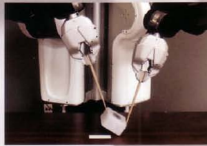
Willow Garage's PR2 robot learns to play billiards and to manipulate chopsticks. The control methods used here, which were developed by Kappens' group, are being implemented by Stefan Schaal at the University of Southern California.
