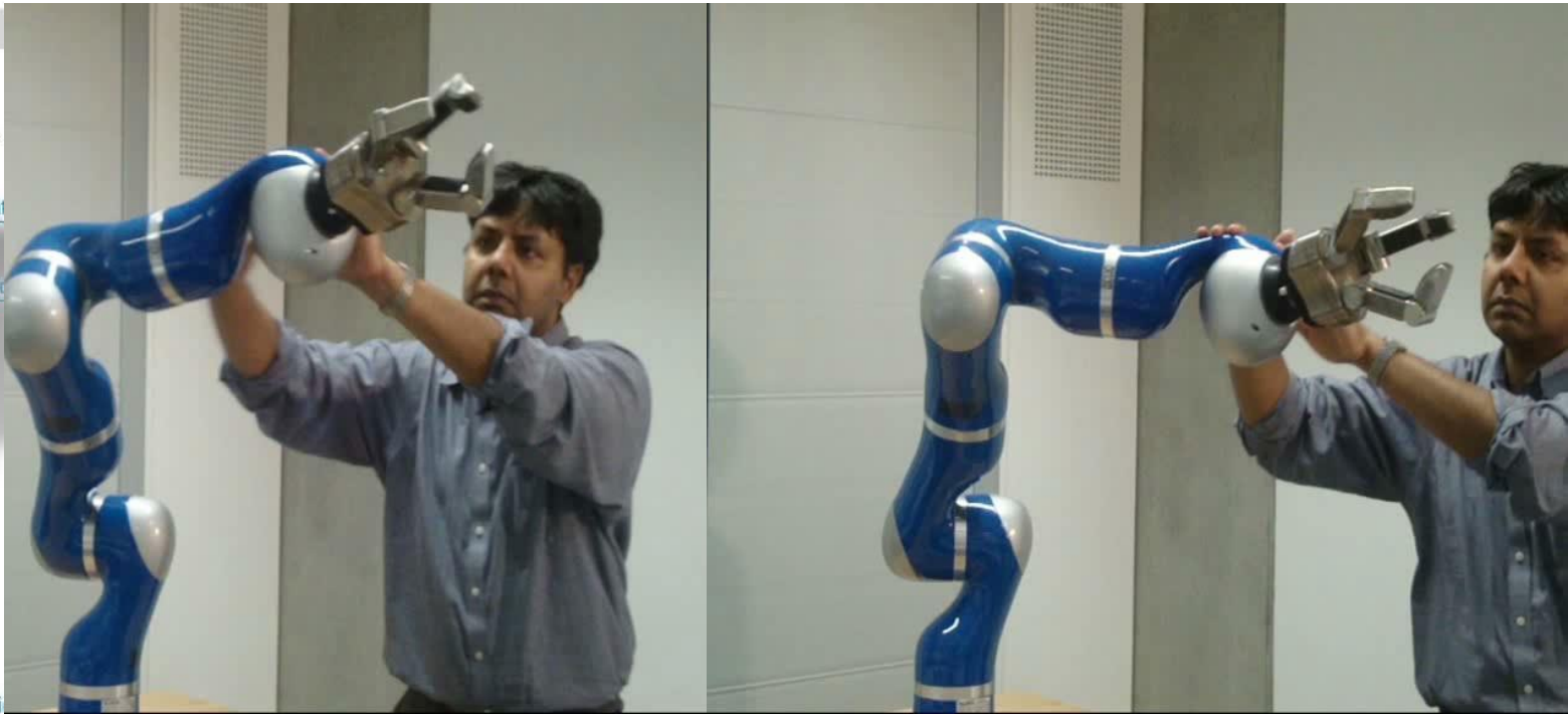
KUKA 7 DOF arm with Schunk 7 DOF hand @ Univ. of Edinburgh
